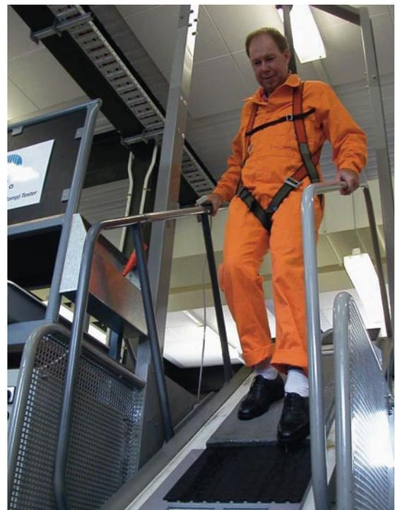
**Figure 2** A ramp test being conducted
